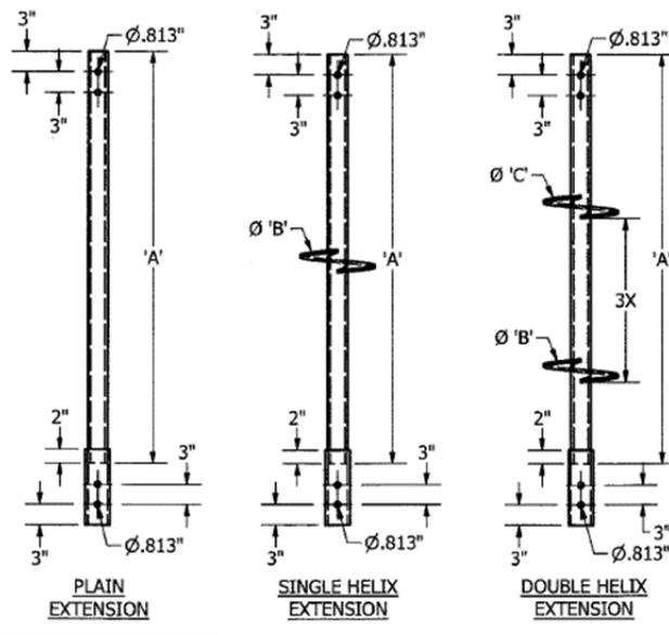
FIGURE 4—TYPICAL 2<sup>7</sup>/<sub>8</sub>-INCH-DIAMETER AND 3<sup>1</sup>/<sub>2</sub>-INCH DIAMETER EXTENSION SHAFT SECTIONS INCLUDING HELIX EXTENSIONS
