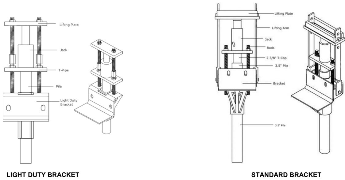
FIGURE 1—FOUNDATION REPAIR BRACKET FOR 2<sup>7</sup>/<sub>8</sub>-INCH-DIAMETER AND 3<sup>1</sup>/<sub>2</sub>-INCH-DIAMETER SHAFTS
