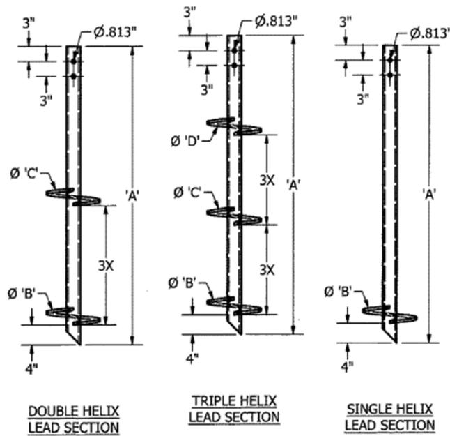
FIGURE 3—TYPICAL 2<sup>7</sup>/<sub>8</sub>-INCH-DIAMETER AND 3 1/2-INCH DIAMETER HELICAL LEAD SHAFT SECTIONS
